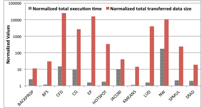
Figure 1: The execution time and transferred data size with OpenACC default memory management scheme. The values are normalized to those for fully optimized OpenACC code.
